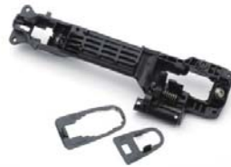
CW-DH-0126 OUTSIDE CAR DOOR HANDLE BASE ONLY FRONT RH/LH TOYOTA RAV4 '01-05 OE# 6920252010 L 6920152040 R
