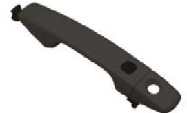
CW-DH-0168 OUTSIDE CAR DOOR HANDLE W/KEY HOLE FRONT TOYOTA LAND CRUISER FJ200 '2007 OE# 6921060100 L 6921060100 R
