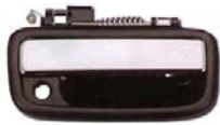
CW-DH-0077 OUTSIDE CAR DOOR HANDLE CHROME RH/LH TOYOTA TACOMA PICK UP '95 OE# 6922035030 L 6921035030 R
